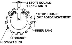
Figure 11 - Locknut Adjustment
