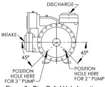
Figure 9 - Disc Relief Hole Location
