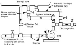
Figure 3 – Bypass Valve Mounting
