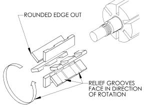
Figure 8 – Vane Installation
