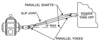
Figure 7 – Pump Drive Note: A Drive Shaft Guard between the pump and the PTO MUST be provided. (Not Shown)
